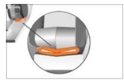
A pump head with convex shaped rollers that does not pinch the tubing in the conventional way is suitable for cell research.
