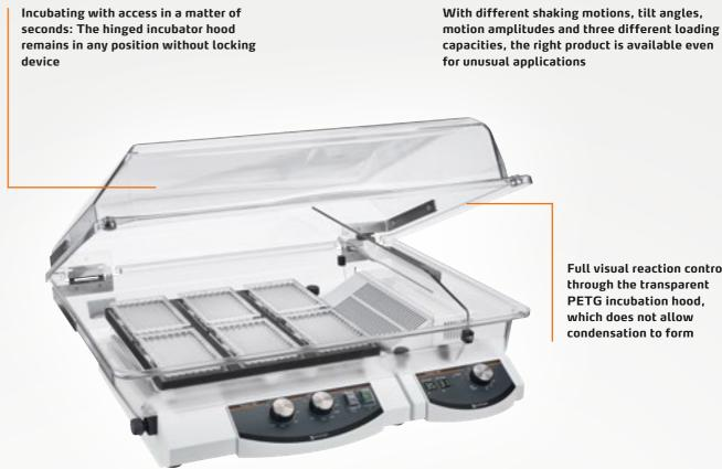
Full visual reaction control through the transparent PETG incubation hood, which does not allow condensation to form
